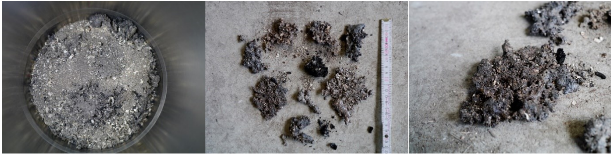
Figure 17: Ash agglomerates in the bottom ash during the combustion of WCB+H in the Endress combustion plant, type USF-W 800.
