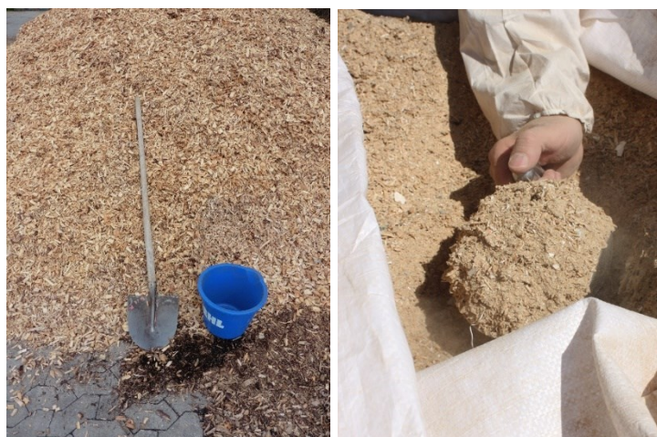
Figure 2: Photos of the raw materials procured within the framework of the project (left: forest residues, right: residues from chipboard processing)
