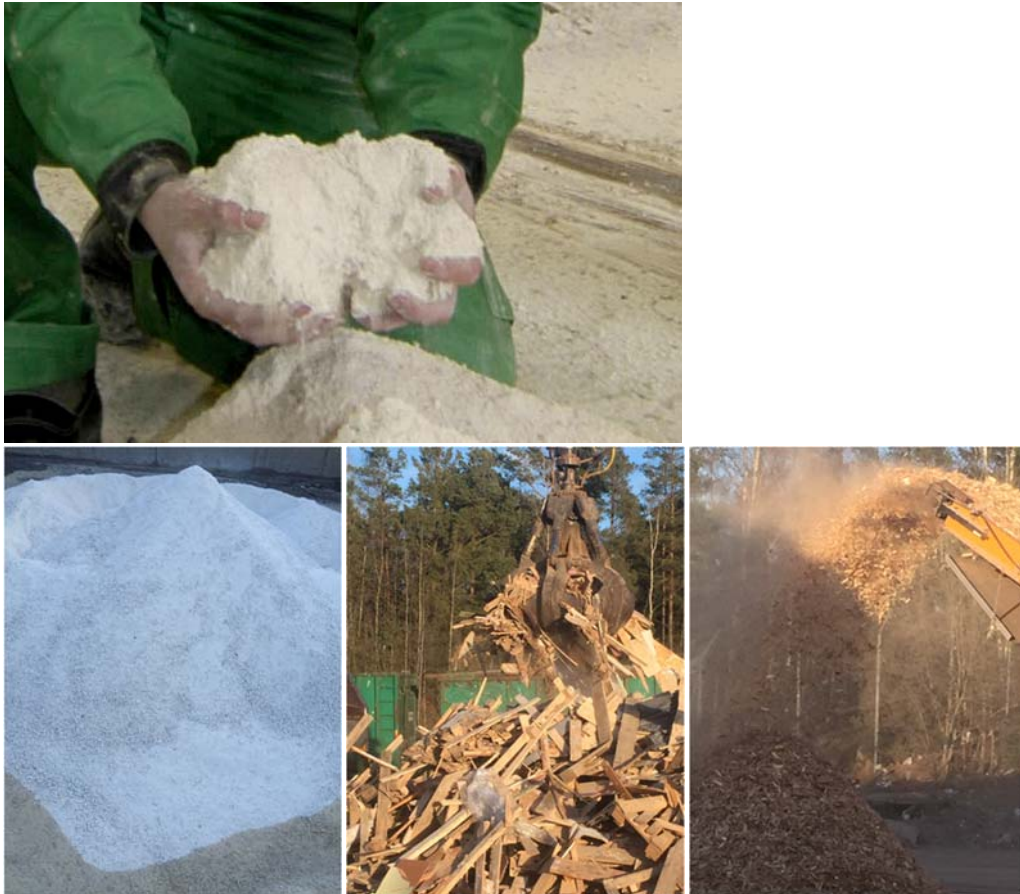
Figure 9: Gypsum additive used in the ENA power plant, mixed with demolition wood
